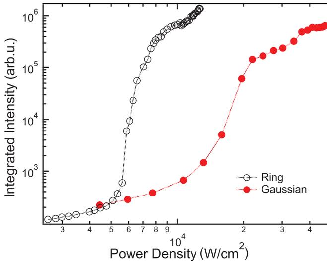
FIG. 4. (Color online) Integrated intensity with increasing power density from the trapped condensate (open black circles) and from a Gaussian excitation (red circles) measured at  $k = 0 \mu\text{m}^{-1}$  of the spatially filtered dispersions.
