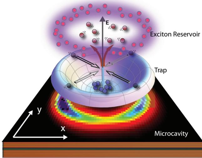
FIG. 1. (Color online) Polariton trap over real-space excitation spot, displaying the trapping mechanism. Polaritons scattered to high-energy states leave the trap, while those scattered to low energy and momentum remain confined.
