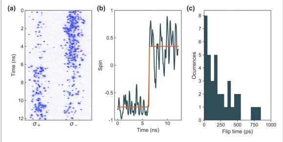
**Figure 4.** Raw streak image showing single-photon events (a) and extracted spin trace (b) of an ultrafast flip with duration  $52\pm1$  ps (c) histogram of fitted flipping duration times.
