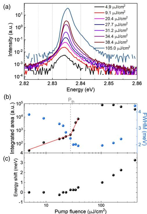
**Fig. 4.** (a) PL spectra at  $k_{\parallel} = 0$  extracted from the angle-resolved PL in Fourier space at different excitation energies. (b) The integrated area of emission spectrum at  $k_{\parallel} = 0$  and the full width at half maximum as functions of pump fluence. The transition from a linear regime to non-linear regime defines the threshold at 27.7  $\mu\text{J}/\text{cm}^2$ . (c) Blue-shift of emission peak as a function of pump fluence.
