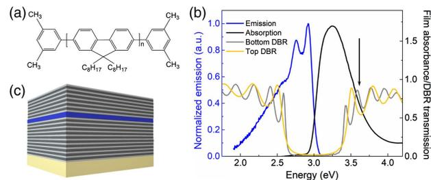
**Fig. 1.** (a) Chemical structure of PFO. (b) Absorption and emission spectra of a 135-nm-thick bare PFO film and transmission of the bottom and top DBRs at normal incidence. The black arrow indicates the excitation wavelength. (c) Schematic of the DBR microcavity.
