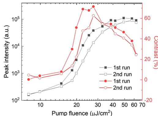
**Fig. 6.** Black solid and open squares, respectively, show the peak photoluminescence intensity of interferograms as a function of pump fluence in the first and second measurements. Red solid and open circles, respectively, show the fringe visibility for increasing pump fluence in the first and second measurements.
