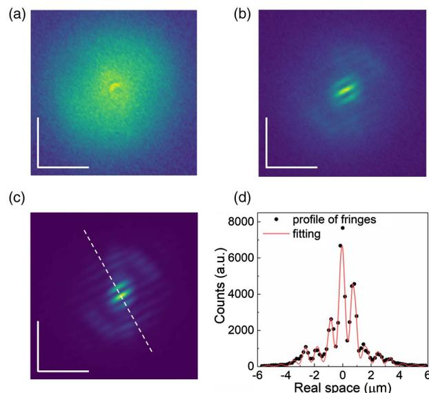
**Fig. 5.** Interferograms recorded in a Michelson interferometer for increasing pump fluence, (a) at 9.9  $\mu\text{J}/\text{cm}^2$ , (b) 18.3  $\mu\text{J}/\text{cm}^2$ , and (c) 27.5  $\mu\text{J}/\text{cm}^2$ . All scale bars are 5  $\mu\text{m}$ . (d) The black solid circles are the intensity profile along the white dashed line in (c), and the red line is the fit (see Section 2).
